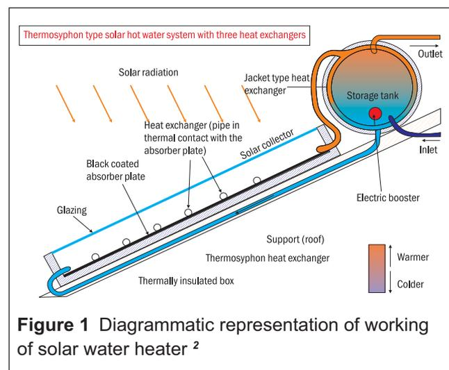
Figure 1 Diagrammatic representation of working of solar water heater <sup>2</sup>
